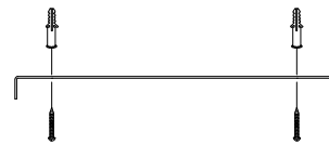
2 Align, mark and drill holes
